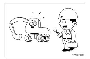
Check for leakage of engine oil, hydraulic oil, fuel and coolant.
