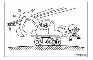
Watch out for obstacles. Be particularly careful to check the machine clearance during the swing.
